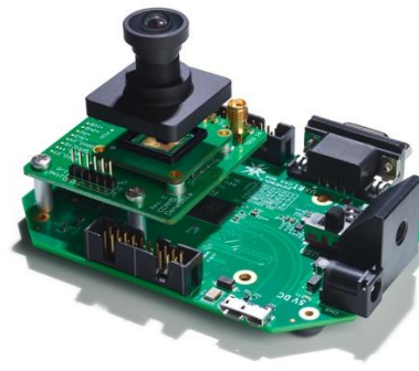
EVK3 mounted with the COB module and an S-Mount optic.
